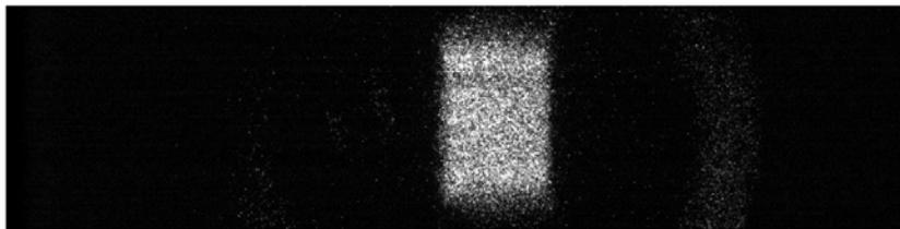
**Figure 3: ICCD image of the homogeneous discharge occurring after the FIW passing**
