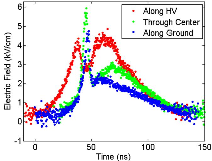
**Figure 1: Temporally resolved electric field measurements at different locations on the plate**
