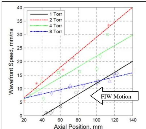
Fig. 1 – Speed of the FIW vs. pressure.
