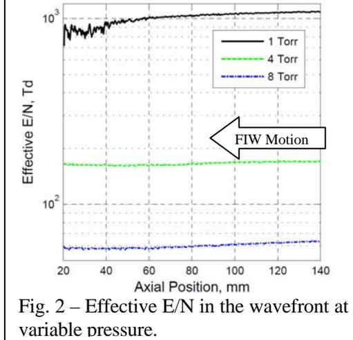
Fig. 2 – Effective E/N in the wavefront at variable pressure.
