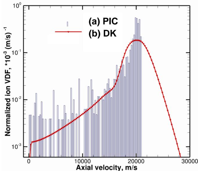
• Ion VDF at the channel exit of a Hall thruster. (a) PIC, (b) DK
