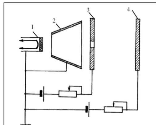
Figure 1 – Schematic of the discharge. 1) Hot cathode, 2) bounding wall, 3) anode, 4) auxiliary electrode.
