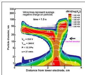
Fig. 1 – Predicted profiles over electrode gap of particle size distribution and average particle charge (white lines), 1.5 s following plasma turn-on.
