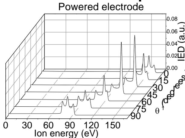
Simulated IEDs on the powered electrode in a 7.5 mTorr Ar CCP.  $U_1=U_2=100$  V,  $f_1=13.56$  MHz,  $n_e=2 \times 10^9$  cm<sup>-3</sup>,  $T_e=3$  eV, and electrode area ratio =2.0.
