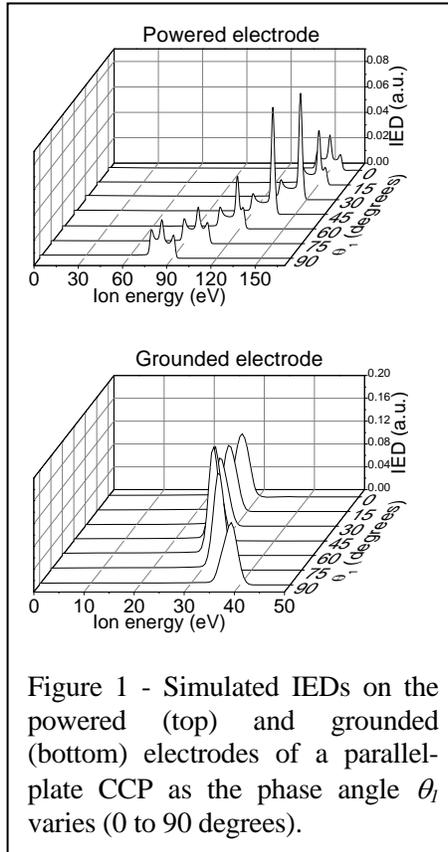
Figure 1 - Simulated IEDs on the powered (top) and grounded (bottom) electrodes of a parallel-plate CCP as the phase angle  $\theta_i$  varies (0 to 90 degrees).
