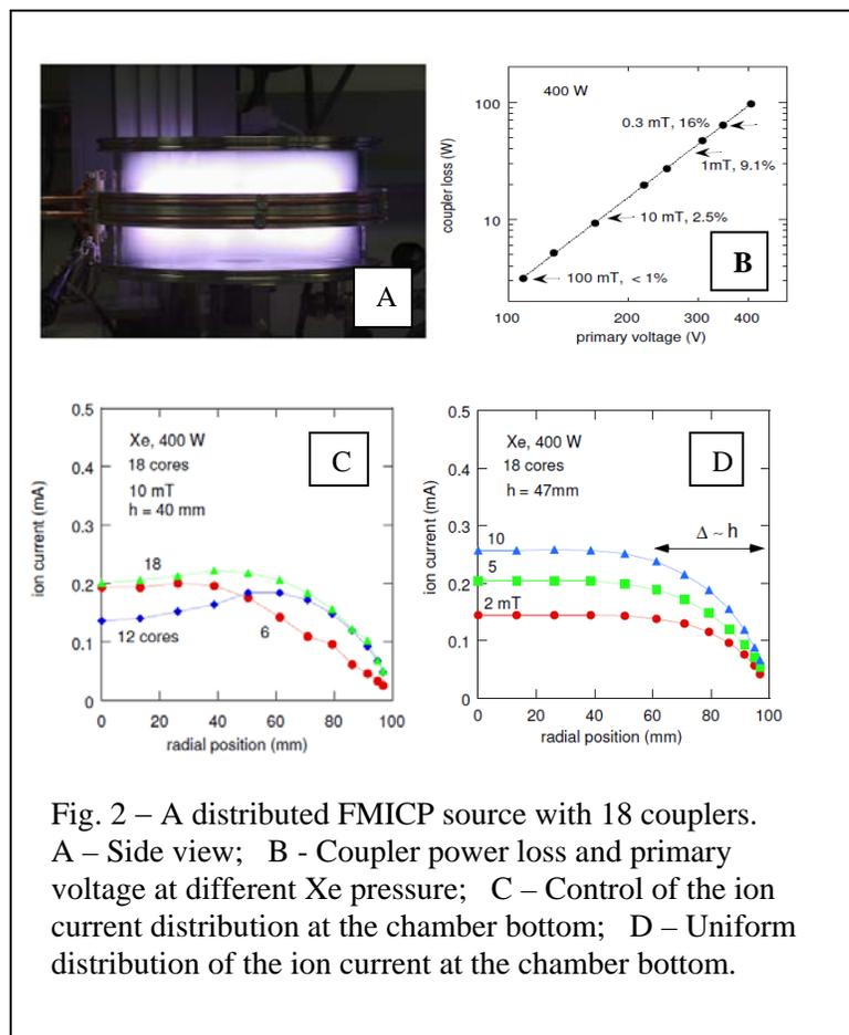
Fig. 2 – A distributed FMICP source with 18 couplers. A – Side view; B - Coupler power loss and primary voltage at different Xe pressure; C – Control of the ion current distribution at the chamber bottom; D – Uniform distribution of the ion current at the chamber bottom.
