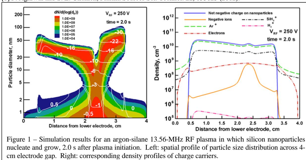
Figure 1 – Simulation results for an argon-silane 13.56-MHz RF plasma in which silicon nanoparticles nucleate and grow, 2.0 s after plasma initiation. Left: spatial profile of particle size distribution across 4-cm electrode gap. Right: corresponding density profiles of charge carriers.
