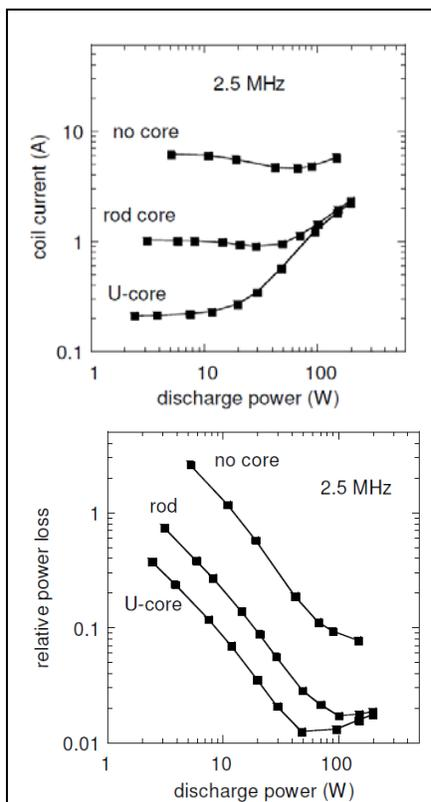
Fig. 1 – Effect of ferromagnetic core on the coupler current (A), and on the coupler power loss (B).
