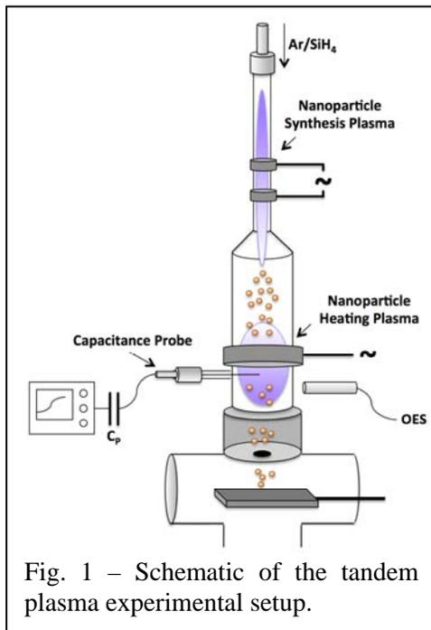
Fig. 1 – Schematic of the tandem plasma experimental setup.
