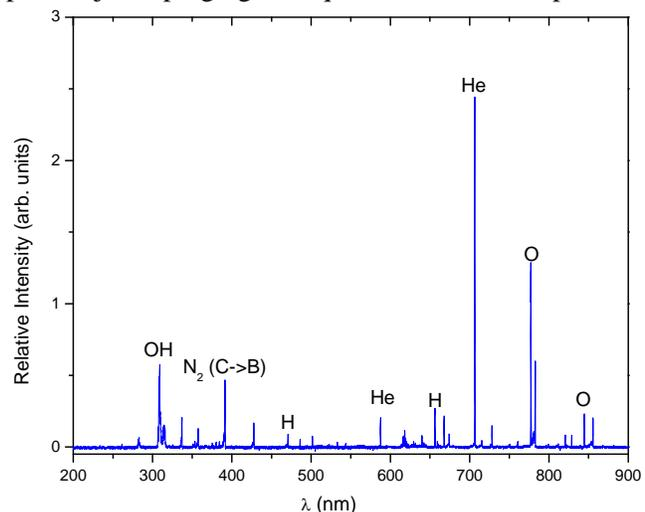
Figure 2 - Optical emission spectrum of a He plasma jet in open air impinging on a quartz window. The spectrum was recorded through the window at an angle of 90° with respect to the surface, sampling the whole plasma.
