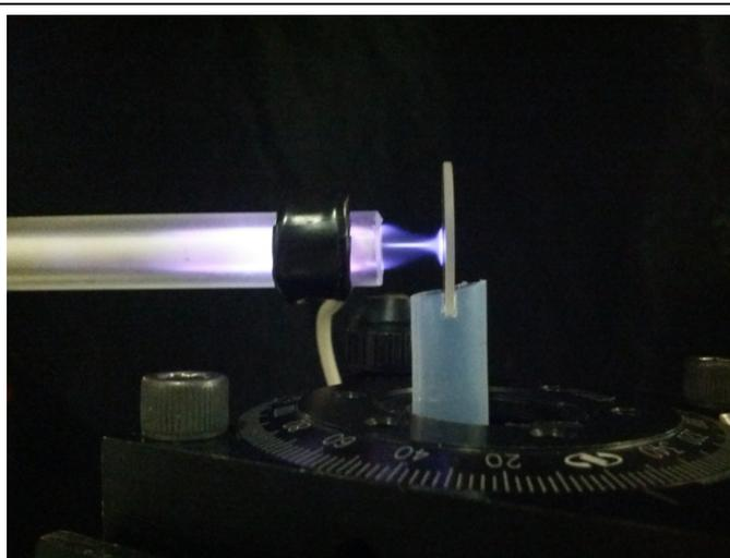
Figure 1 - Photograph of an atmospheric pressure He plasma jet impinging on a quartz substrate in open air.
