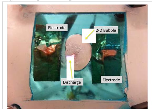
Figure 1 – 2-D bubble with plasma decolorization of Methylene Blue solution.
