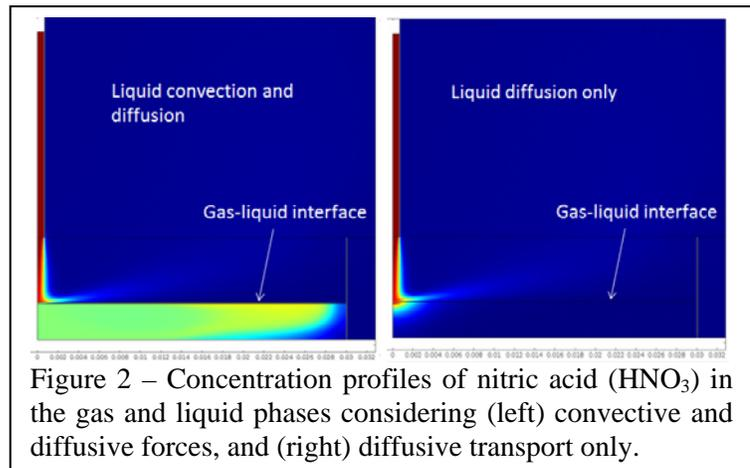
Figure 2 – Concentration profiles of nitric acid ( $\text{HNO}_3$ ) in the gas and liquid phases considering (left) convective and diffusive forces, and (right) diffusive transport only.
