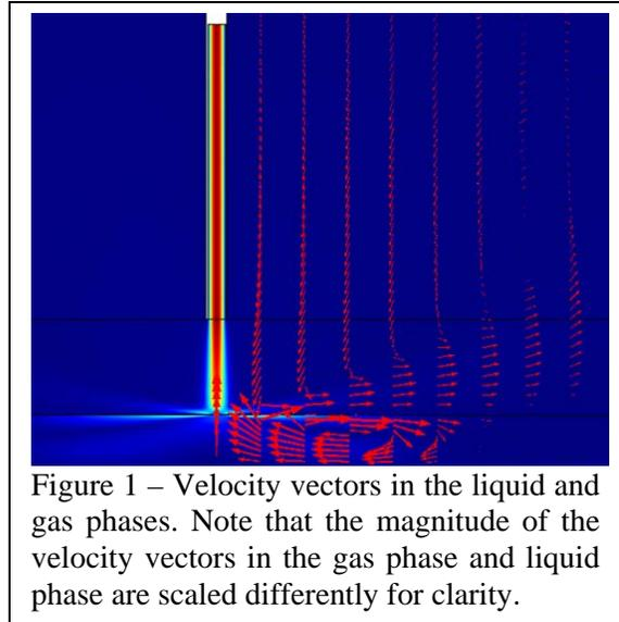
Figure 1 – Velocity vectors in the liquid and gas phases. Note that the magnitude of the velocity vectors in the gas phase and liquid phase are scaled differently for clarity.
