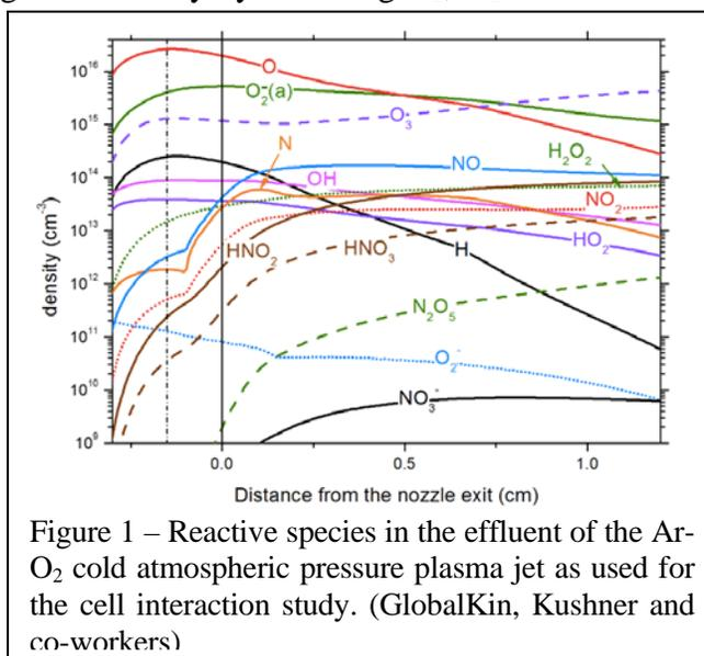
Figure 1 – Reactive species in the effluent of the Ar-O<sub>2</sub> cold atmospheric pressure plasma jet as used for the cell interaction study. (GlobalKin, Kushner and co-workers)
