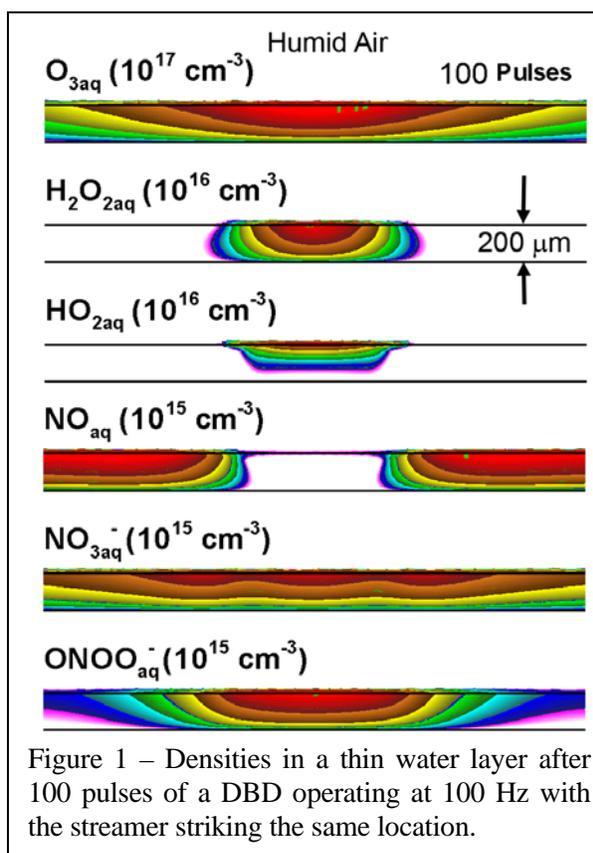
Figure 1 – Densities in a thin water layer after 100 pulses of a DBD operating at 100 Hz with the streamer striking the same location.
