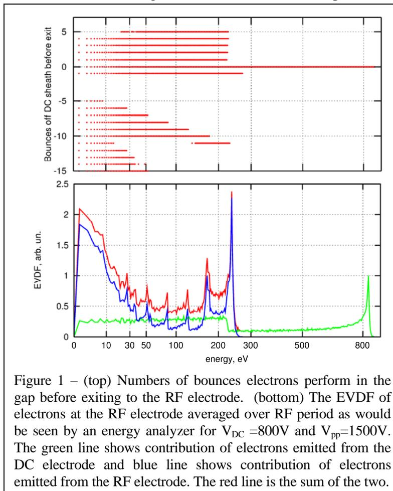
Figure 1 – (top) Numbers of bounces electrons perform in the gap before exiting to the RF electrode. (bottom) The EVDF of electrons at the RF electrode averaged over RF period as would be seen by an energy analyzer for  $V_{DC} = 800V$  and  $V_{pp} = 1500V$ . The green line shows contribution of electrons emitted from the DC electrode and blue line shows contribution of electrons emitted from the RF electrode. The red line is the sum of the two.
