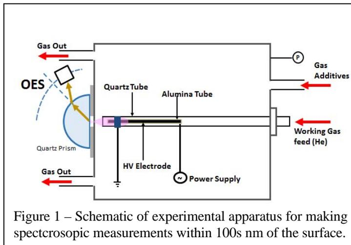
Figure 1 – Schematic of experimental apparatus for making spectroscopic measurements within 100s nm of the surface.
