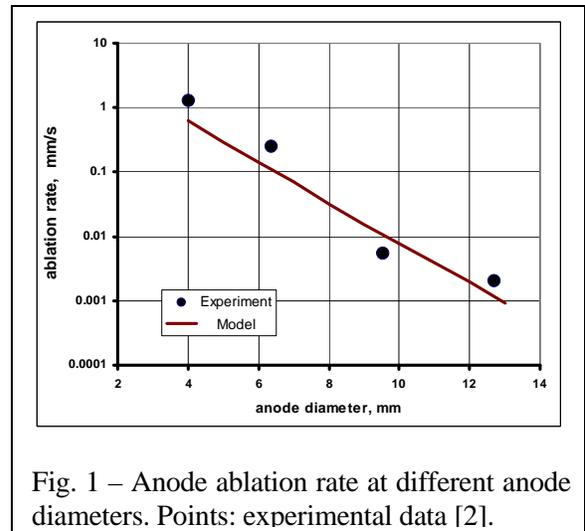
Fig. 1 – Anode ablation rate at different anode diameters. Points: experimental data [2].
