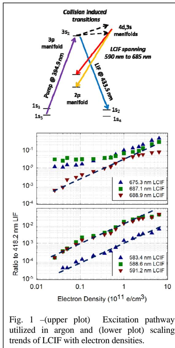
Fig. 1 –(upper plot) Excitation pathway utilized in argon and (lower plot) scaling trends of LCIF with electron densities.
