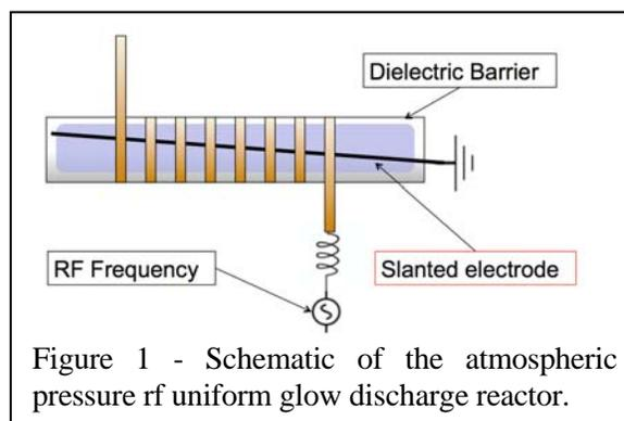
Figure 1 - Schematic of the atmospheric pressure rf uniform glow discharge reactor.
