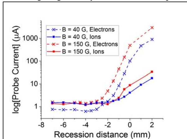
Fig. 1 – Ion and electron currents measured by the MIB probe collector vs recession distances and magnetic field.
