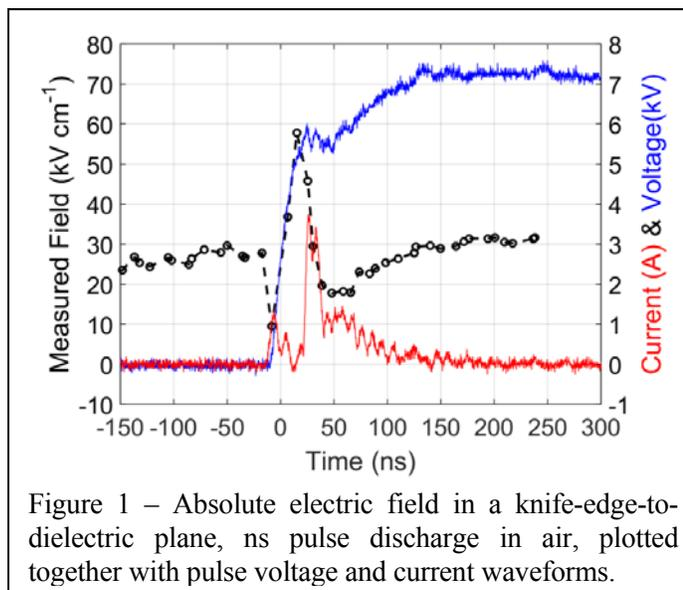
Figure 1 – Absolute electric field in a knife-edge-to-dielectric plane, ns pulse discharge in air, plotted together with pulse voltage and current waveforms.
