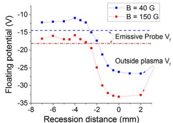
Fig. 2 – Floating potential of the MIB probe. Inside the tube, the collector floats at a potential above that from floating emissive probes.
