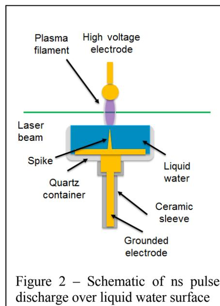
Figure 2 – Schematic of ns pulse discharge over liquid water surface
