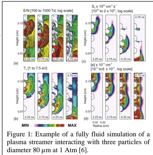
Figure 1: Example of a fully fluid simulation of a plasma streamer interacting with three particles of diameter  $80\ \mu\text{m}$  at 1 Atm [6].
