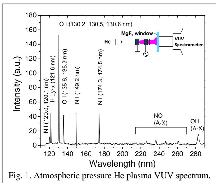
Fig. 1. Atmospheric pressure He plasma VUV spectrum.
