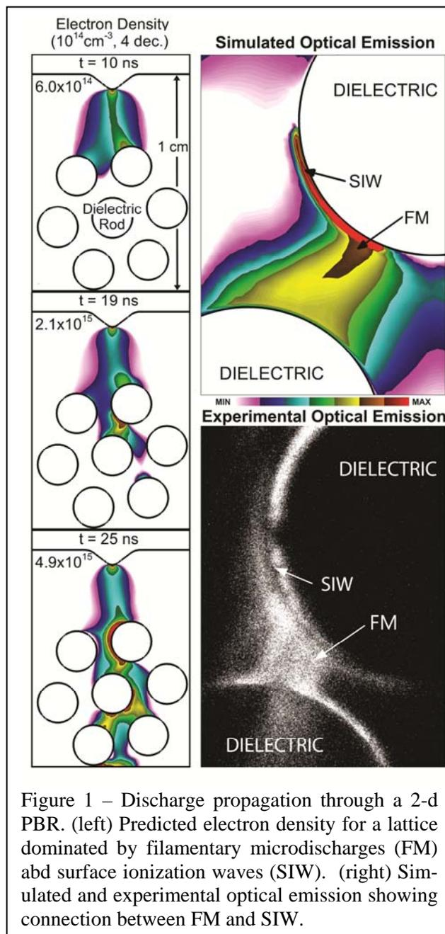
Figure 1 – Discharge propagation through a 2-d PBR. (left) Predicted electron density for a lattice dominated by filamentary microdischarges (FM) and surface ionization waves (SIW). (right) Simulated and experimental optical emission showing connection between FM and SIW.
