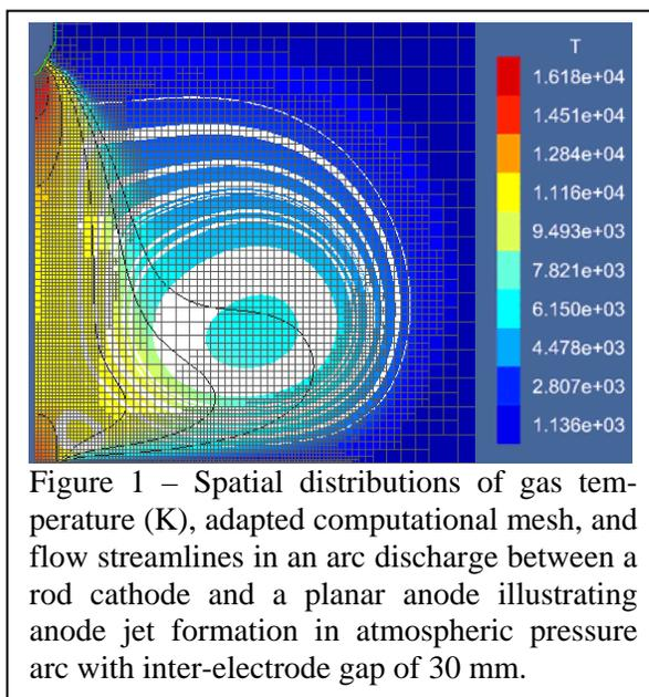
Figure 1 – Spatial distributions of gas temperature (K), adapted computational mesh, and flow streamlines in an arc discharge between a rod cathode and a planar anode illustrating anode jet formation in atmospheric pressure arc with inter-electrode gap of 30 mm.
