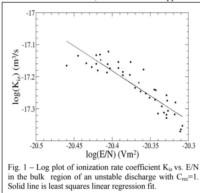
This causes the ionization rate coefficient,  $K_{iz}$ , to decrease with increasing electron temperature  $T_e$  and reduced electric field  $E/N$  in the instability regime. (See Fig. 1). A theoretical instability criterion was developed that showed excellent agreement with the PIC results. We found that discharges with large volume losses (compared to surface losses) tend to be unstable while those with small volume losses tend to be stable.
