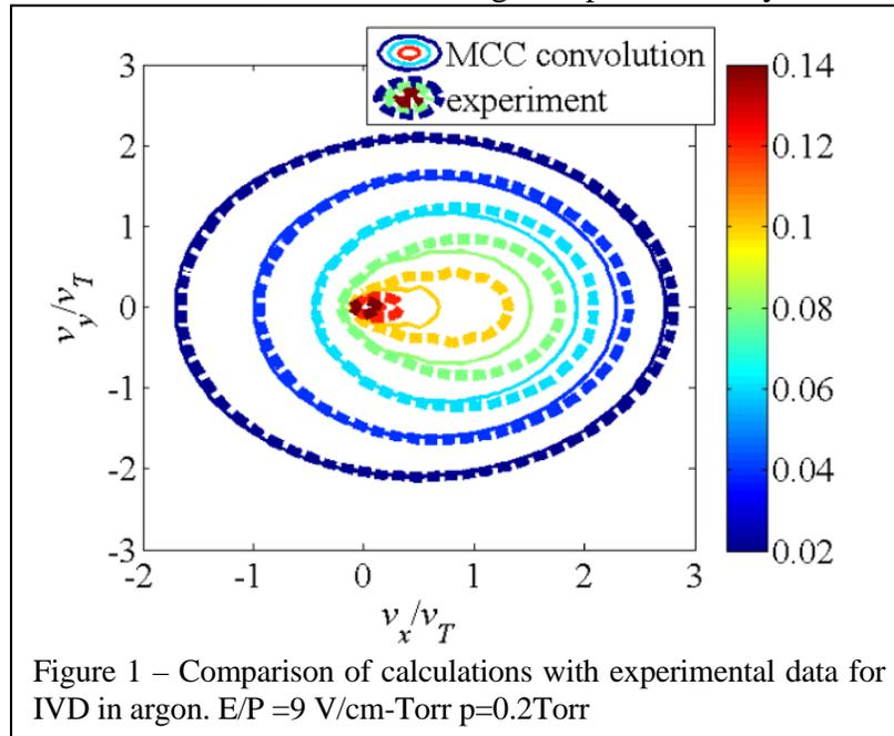
Figure 1 – Comparison of calculations with experimental data for IVD in argon.  $E/P = 9$  V/cm-Torr  $p = 0.2$  Torr
