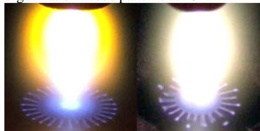
Figure 2 – Plasma emission clouds image with patterns at 2.2kV, 8mm gap length with 200 sccm He flow. *Note: for figures 1 and 2, (L) NaCl solution. (R)  $\text{CuSO}_4$  solution.*
