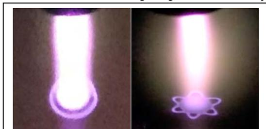
Figure 1 – Different shapes of self-organization anode patterns at 40 mA.
