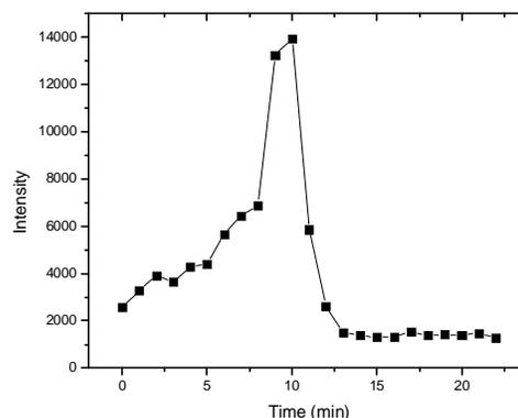
Fig. 1 – OH (309 nm) emission intensity vs. time for an APPJ interacting with a thin water surface film.
