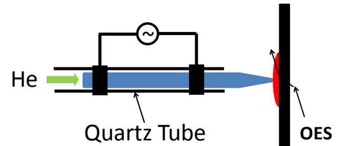
• Fig. 1. APPJ interacting with liquid thin surface film.
