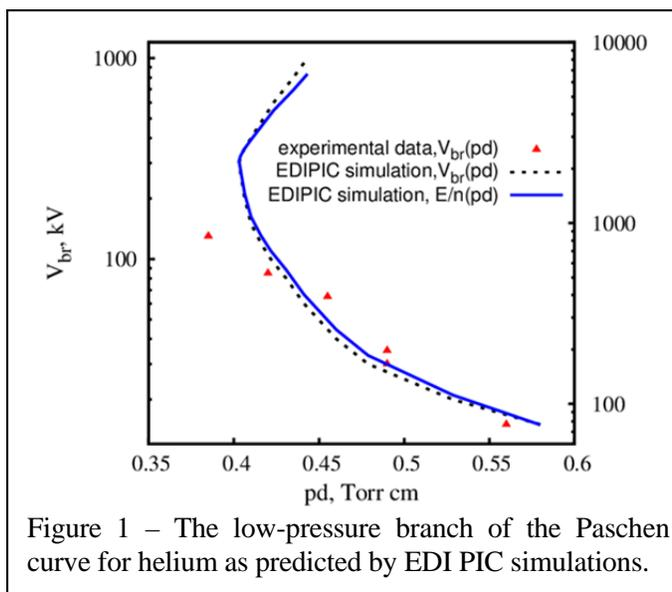
Figure 1 – The low-pressure branch of the Paschen curve for helium as predicted by EDI PIC simulations.
