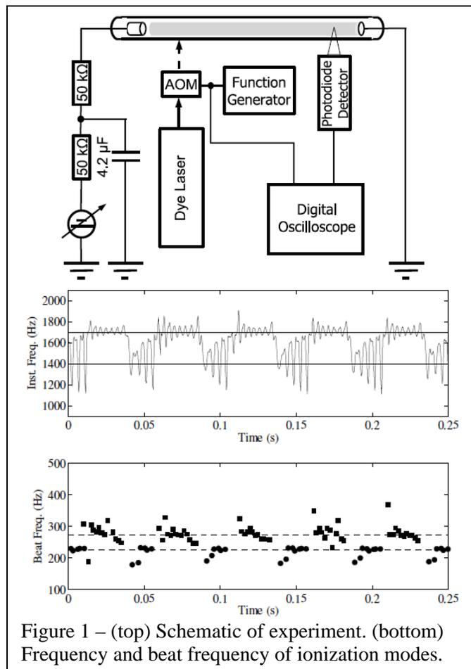
Figure 1 – (top) Schematic of experiment. (bottom) Frequency and beat frequency of ionization modes.
