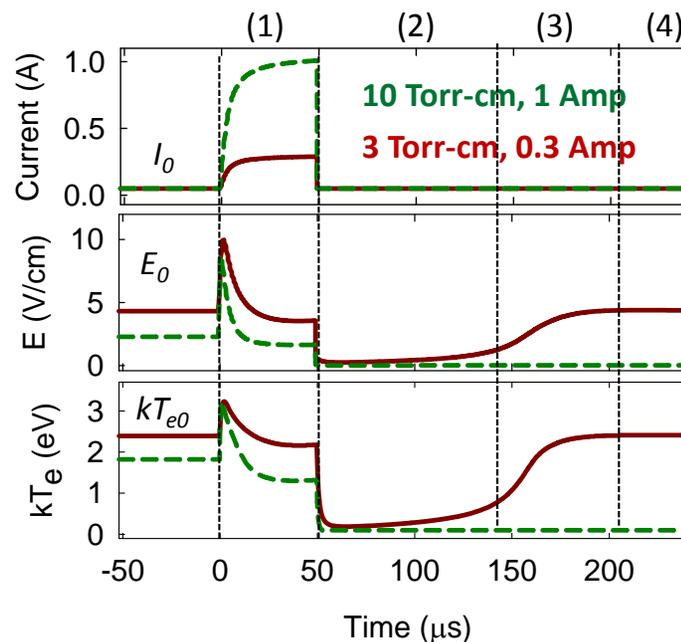
Simulation: Different Stages of Positive Column in Pulsed Current Regimes
