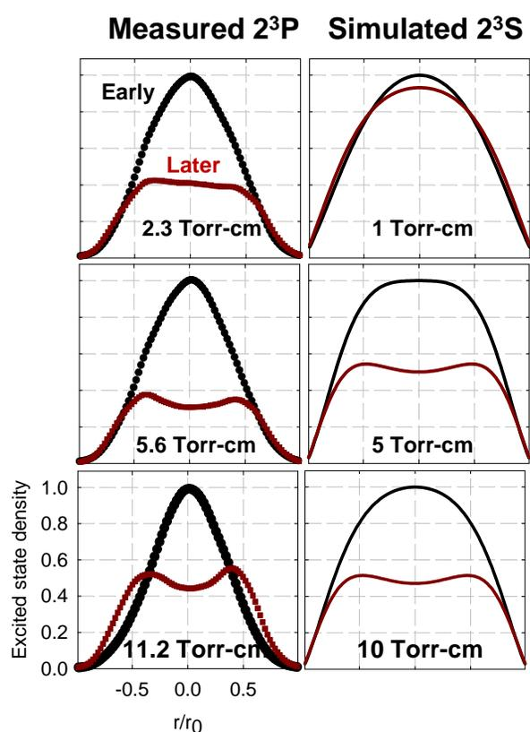
Radial distribution of excited atoms for different pressure and time during the current pulse.
