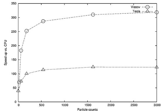
**Fig. 2** Speed up comparison using a particle simulation test case. 300 times acceleration was observed using “Vlasov” computer.
