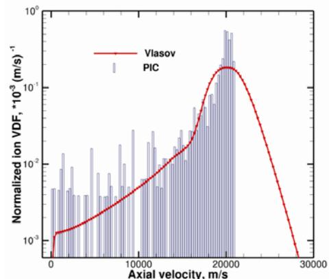
**Fig. 1** Ion VDFs obtained from Vlasov and PIC simulations in the Hall thruster discharge plasma. No statistical noise observed from Vlasov solver.
