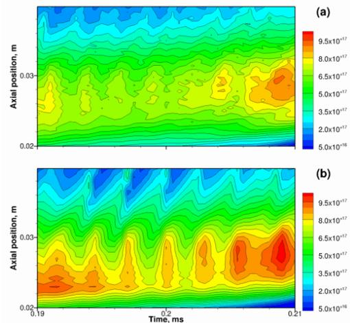
**Fig. 1** Spatial and temporal evolution of the ion number density in the Hall thruster discharge channel: (a) hybrid-PIC (b) hybrid-DK
