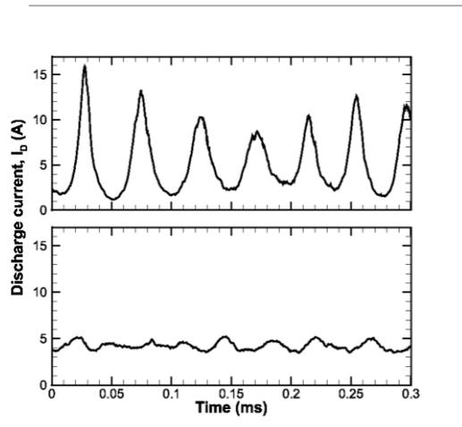
**Fig. 1** SPT-100 thruster 1D hybrid-DK simulation. (top) Global oscillation at 5-30 kHz when magnetic fields are small, (bottom) Local oscillation when magnetic fields are large
