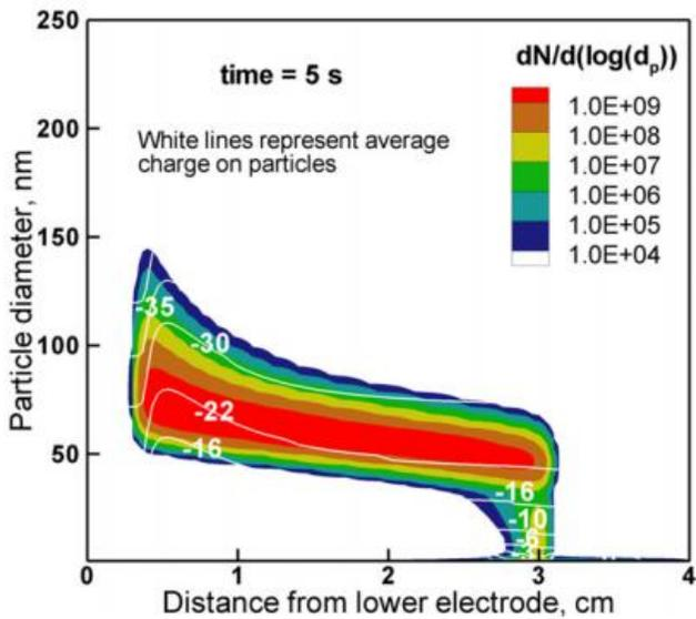
Figure 1 Particle size distribution and average particle charge at  $t = 5$  s
