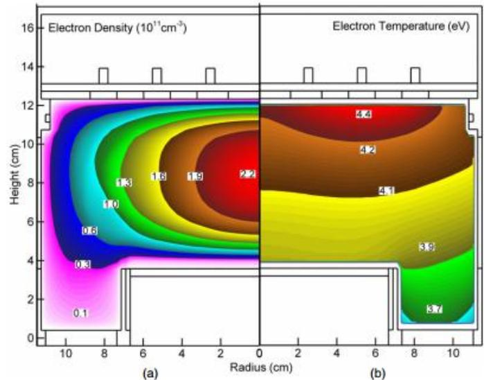
Figure 2 Plasma properties for an Ar/C<sub>4</sub>F<sub>8</sub> ICP with a CCP bias on the substrate. (a) Electron density and (b) electron temperature
