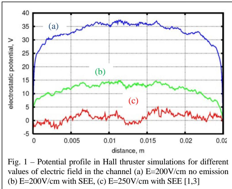
Fig. 1 – Potential profile in Hall thruster simulations for different values of electric field in the channel (a)  $E=200\text{V/cm}$  no emission (b)  $E=200\text{V/cm}$  with SEE, (c)  $E=250\text{V/cm}$  with SEE [1,3]
