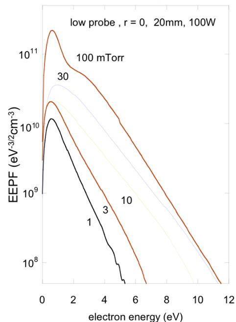
**Fig.5:** Electron energy probability function on the axis, below the coil, with magnet on.
