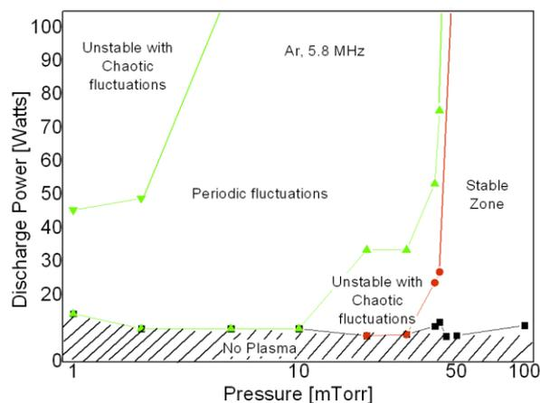
**Fig. 2:** Instability map in the pressure/power domain; with dipole magnet.
