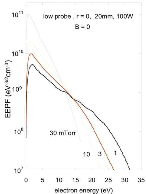
**Fig.4:** Electron energy probability function on the axis, below the coil, without magnet.
