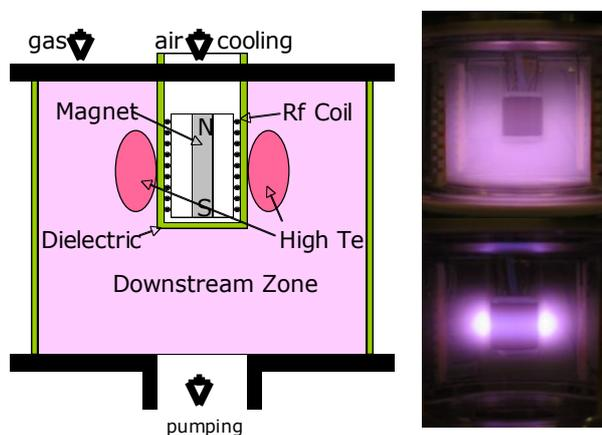
**Fig. 1:** Schematic of the system. A permanent magnet may be added inside the inductive coil to produce a magnetic confinement. Two pictures are taken on the side without magnet (top) and with magnet (bottom), showing the localisation of the plasma when the magnet is on.
