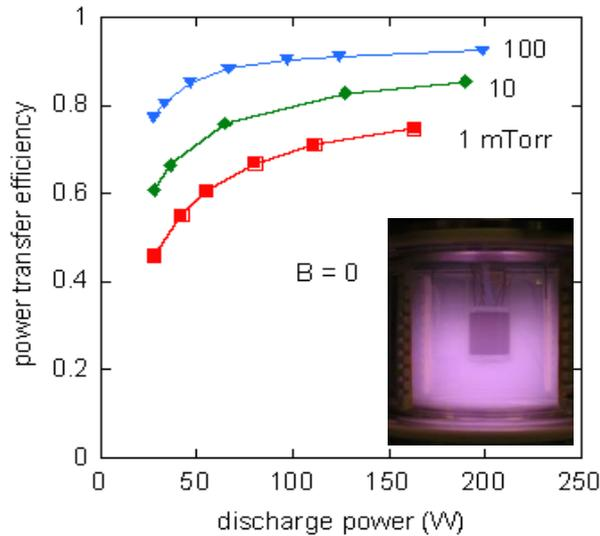
**Fig. 3:** Power transfer efficiency as a function of discharge power without central magnet.
