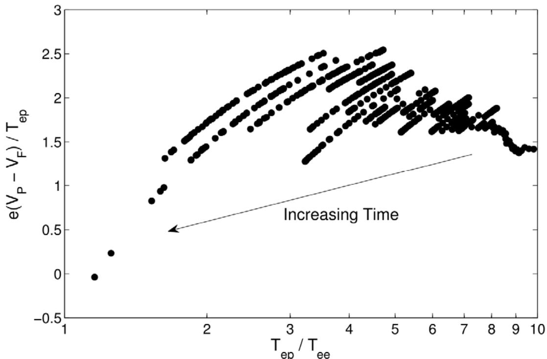
Figure 1: Normalized sheath potential versus plasma to emitted electron temperature ratio
