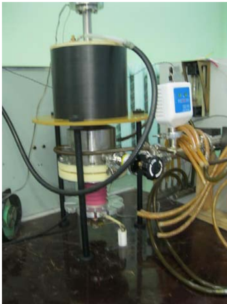
Pulsed B: up to 28 T in 2-3 milliseconds
